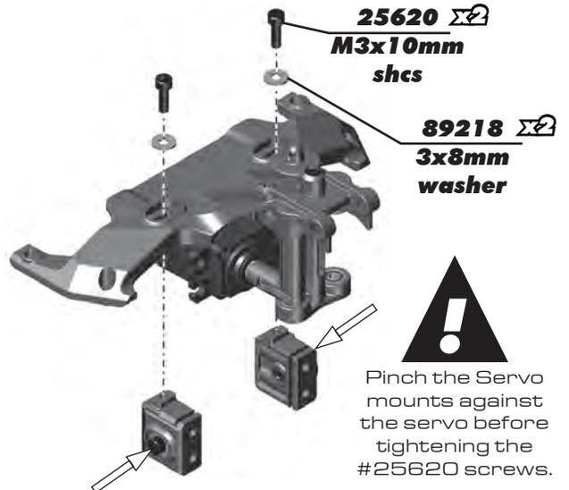
**Pinch the Servo mounts against the servo before tightening the #25620 screws.**
